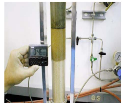
When a cement slurry is placed on top of Ultra Spacer™, no cement filtrate invasion nor additional invasion of Ultra Spacer™ is observed after 46 minutes.*
