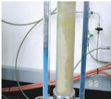
Filtrate from a cement slurry penetrates untreated dry, 20/40-mesh sand in less than 1 minute.*
