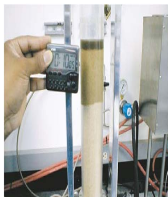
Ultra Spacer™ penetrates untreated sand to a depth of 4 inches before creating a seal.*
